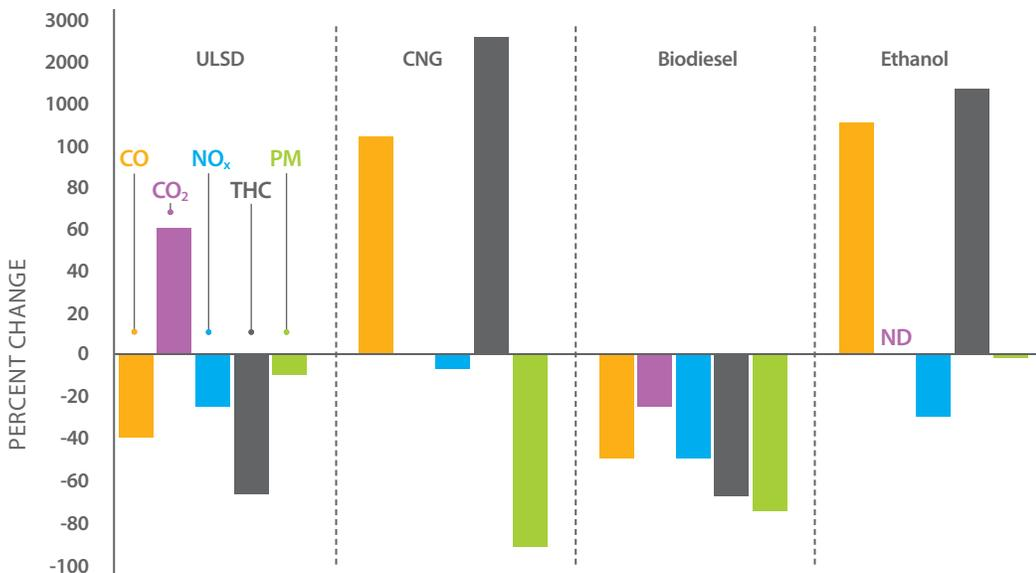
**Figure 3b** Percent Change in Mean Emissions for ULSD with Technologies Compared to ULSD
