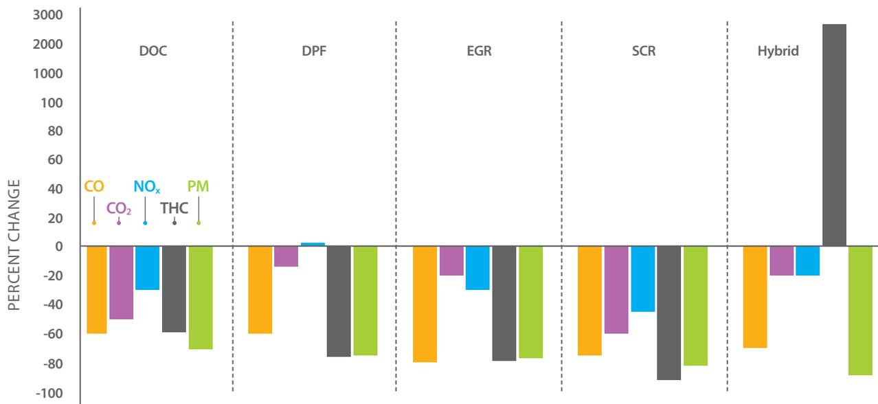
**Figure 3c** Percent Change in Mean Emissions for CNG with Technologies Compared to CNG
